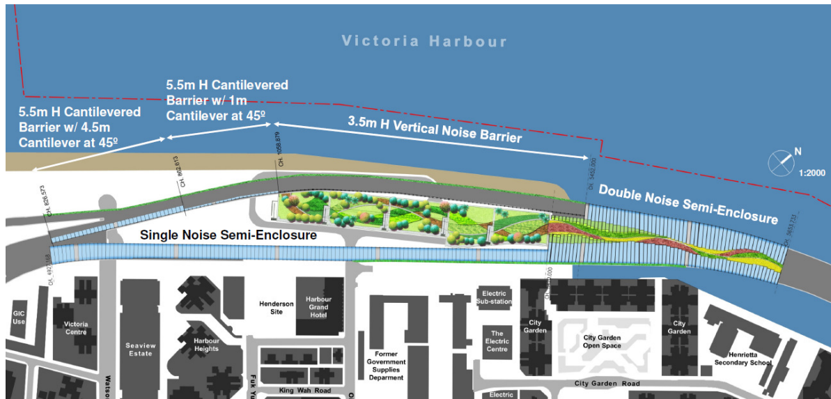
Figure 1 – Extent of Green Wall Panel of Cantilever Noise Barrier at New Eastbound Bridge
